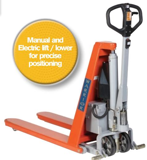
All **WARRIOR** High Lift Pallet Trucks will work happily with open bottomed pallets eg europallets and stillages. They will not work with "Full Perimeter Board" Pallets. Scissor pallet trucks aid manual handling and are a useful truck to have around any factory.
