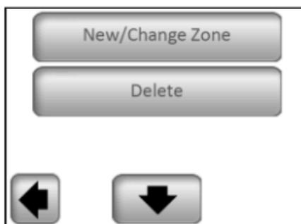
The “**New/Change Zone**” zone button enables new zones to be added or current zones to be altered/changed. The pairing procedure is described in Chapter 2.3.
