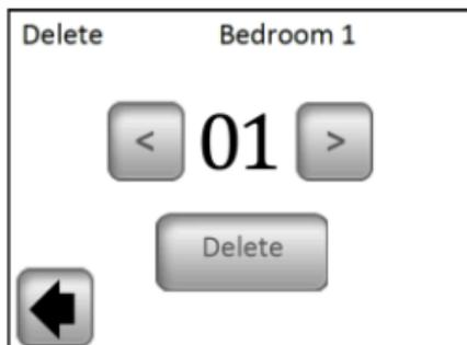
Select the zone to be deleted using the (<) or (>) buttons and press the “**Delete**” button. Confirmation of the deletion by pressing the
