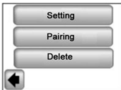
1. Switch the auxiliary RF antenna of your GSM module to the pairing mode (RF init) by pressing the RF button for a period of 3 seconds. The LED diode on the antenna will start glowing green. Now press the “**Pairing**” button on your central unit and the pairing of both units will take place.
