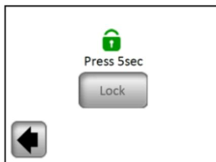
The locking of the display is signalled by a red padlock icon. You can activate the display by pressing this icon for a period of 5 seconds.
