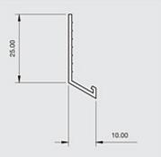
Locally manufactured from recycled plastic, Renderplas PVC stop beads are designed for function and speed on all external and internal rendering and plastering applications. This lightweight profile is designed for external wall insulation and timber frame with thinner renders and where backgrounds are even
