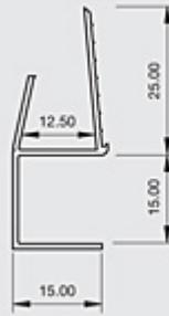
Locally manufactured from recycled plastic, Renderplas PVCu architrave shadow gap beads are designed for plasterboard to quickly and accurately form a shadow gap and provide a superior clean finish. Used at the edges of the plasterboard next to door frames, ceilings and skirting boards where the adjacent finish is hidden
