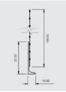
Renderplas PVC EWI and thin coat render stop beads with glass fibre reinforcement mesh. Designed to give maximum speed of installation and add strength to render and EWI systems where render terminates
