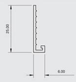
Locally manufactured from recycled plastic, Renderplas PVC small wing stop beads are designed for economy and speed on external and internal rendering and plastering applications where the substrate is even
