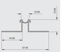
Locally manufactured from recycled plastic, Renderplas PVCu movement joint beads / expansion joints are designed for areas of render over 20 square metres and should be specified every 4-6 metres, over structural movement joints and changes of background. Discreet but strong, all beading gives a perfect finish to through colour render and is equally suitable for sand and cement
