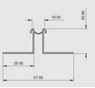
Locally manufactured from recycled plastic, Renderplas PVCu movement joint / expansion joint beads are designed for areas of render over 20 square metres and should be specified every 4-6 metres, over structural movement joints and changes of background. Discreet but strong, all beading gives a perfect finish to through colour render and is equally suitable for sand and cement
