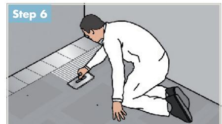
Ready to lay tiles: apply a complete bed of flexible tile adhesive (class C2/S1 acc. EN 12004/12002), in accordance with manufacturer's guidelines.
