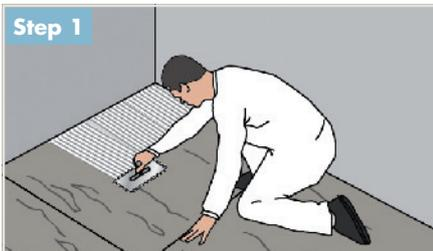
Apply a complete bed of flexible tile adhesive (class C2/S1 acc. EN 12004 /12002) to the subfloor, in accordance with manufacturer's guidelines. Wooden subfloor must be primed before applying Knauf AQUAPANEL® Cement Board Floor Tile Underlay.
