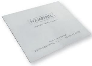
Aggregated Portland cement board with coated glass fibre mesh embedded in back and front surfaces. The ends are square cut and the edges reinforced and finished smoothly (EasyEdge™).
