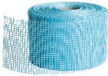
Knauf AQUAPANEL® Tape is a 100mm wide glass fibre tape with an alkaline-resistant coating. It is embedded into AQUAPANEL® Joint Filler and Skim Coat – White, or tile adhesive, to reinforce joints as part of a Knauf AQUAPANEL® Interior system.
