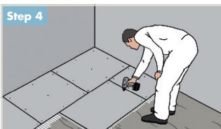
Nine screws per board evenly distributed with a minimum distance from the board edge of 15mm.
