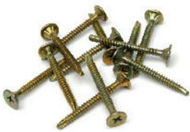
Knauf AQUAPANEL® Maxi Screws have been specifically developed for fixing Knauf AQUAPANEL® Cement Board Indoor onto timber and metal framework of differing thicknesses. Both needlepoint (SN) and drillpoint (SB) versions with countersunk heads are available.
