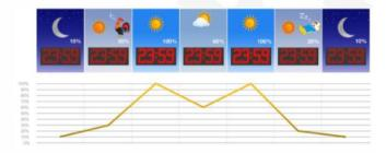
Current measurement by the sensor is always up-to-date, because it takes into account changes of the position of the Sun in relation to the display, changes of cloud cover during a day, and also shortening and lengthening of a day during a year.
