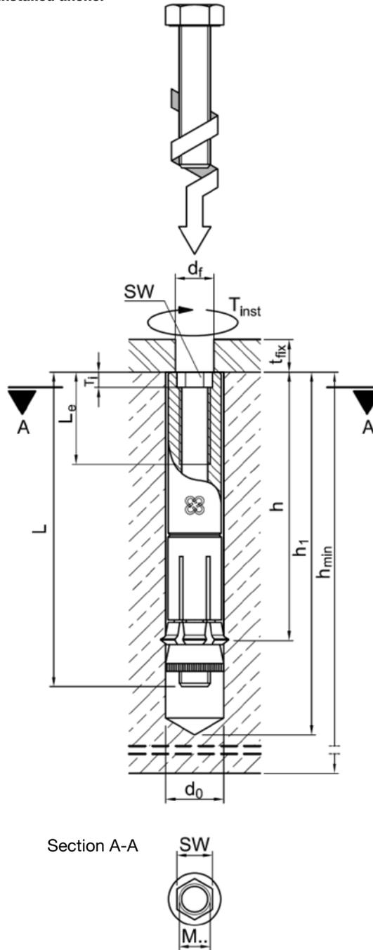
1) The permissible loads have been calculated assuming that grade 8.8 fasteners are used and using the partial safety factors for resistances stated in ETA-01/0011 and a partial safety factor for actions of  $\gamma_F = 1.4$ . The permissible loads are valid for unreinforced concrete and reinforced concrete with a rebar spacing  $s \geq 15$  cm and reinforced concrete with a rebar spacing  $s \geq 10$  cm if the rebar is 10 mm or smaller.
