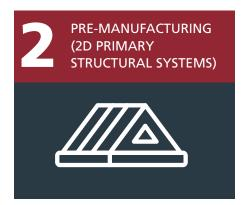
This approach uses flat panel units used for basic floor, wall and roof structures of varying materials, which are factory produced and assembled onsite to create a final three-dimensional structure. The most common approach is to use open panels, or frames, which consist of a skeletal structure only. Services, insulation, external cladding and internal finishing are usually installed onsite.
