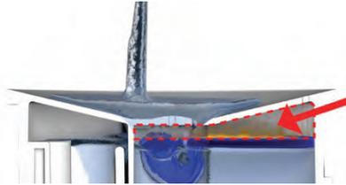
Odour can accumulate in this cavity
