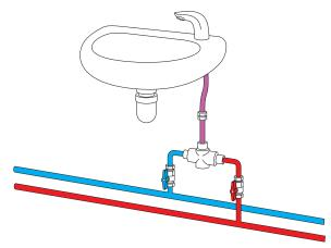
**Single Supply - Pre-mixed:** No-touch basin tap with single pre-mixed water supply using seperate thermostatic mixing valve
