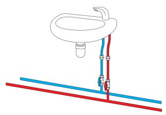
**Hot and Cold Supply - Preset Temperature:** No-touch basin mixer tap with preset temperature (non-thermostatic)
