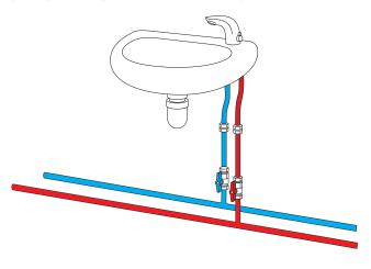
**Hot and Cold Supply - Adjustable Temperature:** No-touch basin mixer tap with temperature adjustment control (non-thermostatic)
