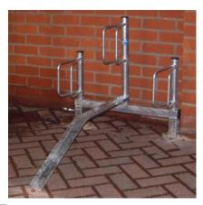
The VELOPA Type B Cycle Rack is a floor mounted cycle rack based upon the Model R Holder. The Type B offers a high single sided cycle parking density. The high and low holders combined ensure that cycles are parked only 305mm apart (typical parking distance for a Sheffield Cycle Stand is 500mm). The high holders, which incorporate ramps are alternated with the low holders, ensuring that all holders can accomdate bicycles at the same time at a higher density than single level cycle parking racks.
