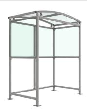
The Burbank shelter is a free-standing, open fronted shelter designed for on site assembly, constructed from galvanised mild steel. Complete with a 4mm PETG clear sheet roof, and ½ side panels. Side-to side curved roof.
