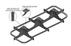
The AUTOPA 'HVM S2 SEAT' is manufactured from Mild Steel and Wood, the steel frame has been galvanised to protect the steel from corrosion.
