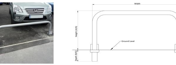
Perimeter Barriers are designed to help secure site perimeters and provide a permanent obstacle to vehicle access, to mark boundaries, define trolley parks and protect vulnerable door entrances and exits.
