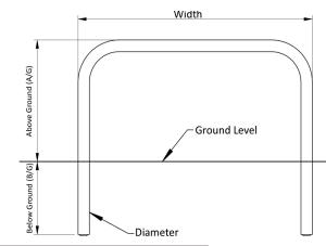
Perimeter Barriers are designed to help secure site perimeters and provide a permanent obstacle to vehicle access, to mark boundaries, define trolley parks and protect vulnerable door entrances and exits.
