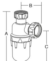
■ Resealing function to prevent loss of water seal
