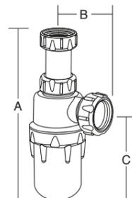
■ Adjustable inlet for installation flexibility
