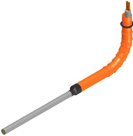
Fig. 05-20 Building entry in a duct in case of buildings with no basement
