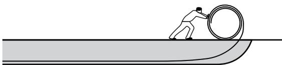
Fig. 07-5 Schematic illustration of open trench installation
