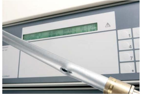
Fig. 03-8 Burst pressure test
