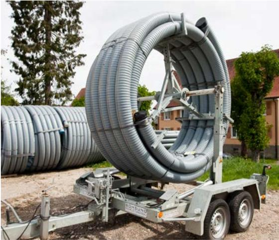
Fig. 07-36 Vertical mobile decoiler
