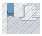
Tests by independent institutes have proved that ISO-BLOCO ONE in dimension 64/3 – 18 mm achieves an evaluated joint sound insulation value of up to 63 dB (-2; -5) in a non-plastered 18 mm joint.
