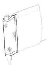
Post & Panel Termination (PPT) -Sleeve slides over post, fabric panel is buried in the bank and attached to end of *Silt Curtain* (up to 100mm dia post, not supplied)
